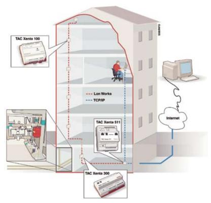
The TAC Xenta 511 allows an operator to easily view and control the devices in a LonWorks network via Internet or local intranet.
