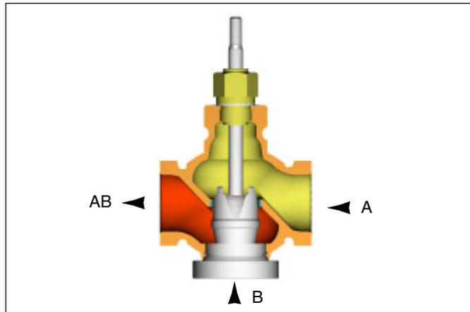
The flow characteristics A - AB of the V341 is equal percentage modified. This characteristic makes it possible to control low flow rates down to almost closed position.
