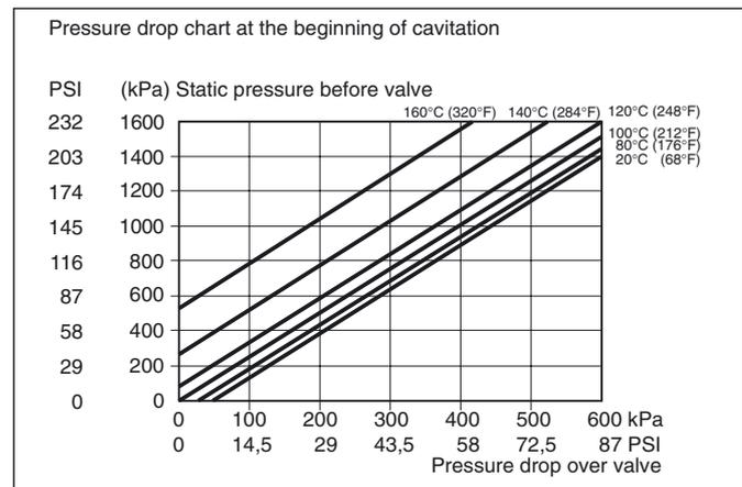
Pressure drop limit where cavitation might occur. Is dependent of valve inlet pressure and temperature of water.
