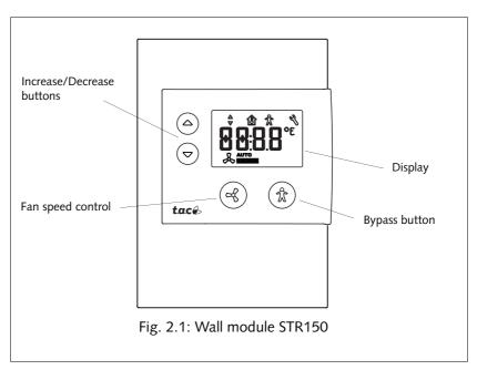
STR150 is connected to TAC Xenta 104-A using two or three wires; the third wire is used if mode indication in the LCD is required. On the other two wires information is sent from the wall unit to the controller:
