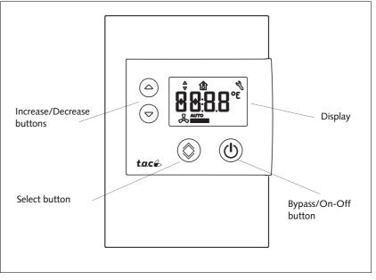
STR350/351 communicates over LonWorks. LonWorks is used for all data exchanges between the room unit and the controller.
