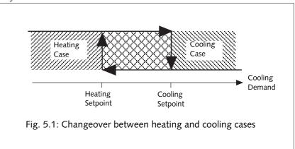
You can force the controller to heat only or cool only, just as you can force it to neither heat nor cool, and to run the fan only. This is achieved using *nviApplicMode*, see Table 5.2, "The relation between nviApplicMode and forcing.".
