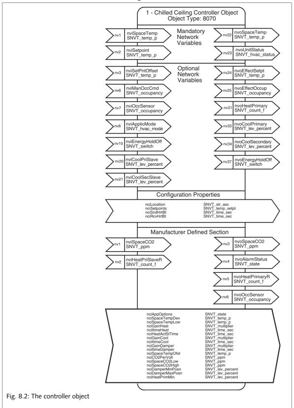
Note! The network variables' indexes are not the same as the figure in "nv" in the diagram below.
