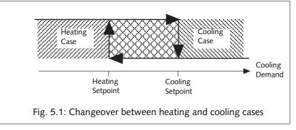
You can force the controller to heat only or cool only, just as you can force it to neither heat nor cool, and to run the fan only. This is achieved using *nviApplicMode*, see Table 5.2, "nviApplicMode".
