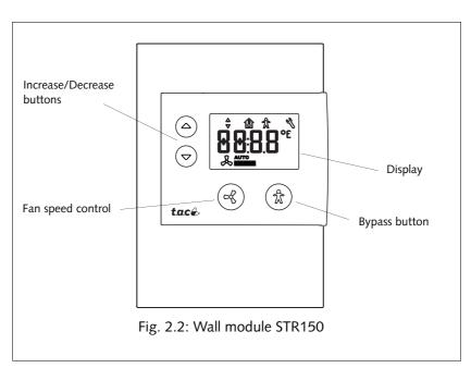
STR150 is connected to TAC Xenta 103-A using two or three wires; the third wire is used if mode indication in the LCD is required. The other two wires are used to send information from the wall unit to the controller:
