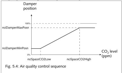
The air flow is set to the highest value of the value from the air quality control and the cooling controller according to figure.
