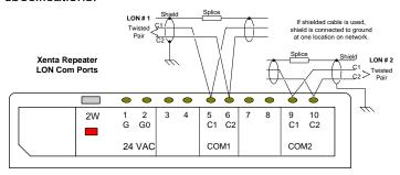
If no Router is present, up to three Repeaters may be used to extend the network channels range. If Routers are used, a maximum of one Repeater is allowed between any two Routers.
