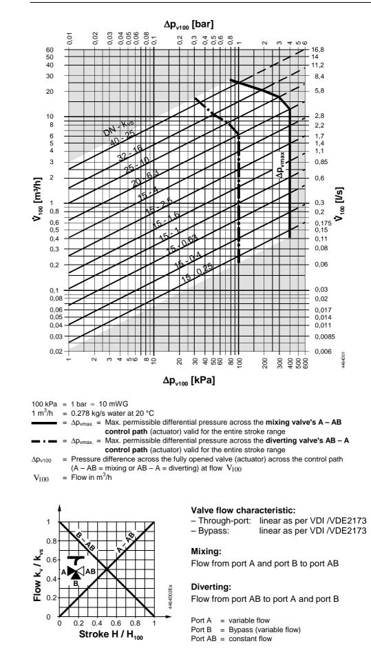
Use the three-port valve primarily as a mixing valve
