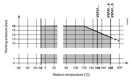
Working pressure and medium temperature staged as per ISO 7005
