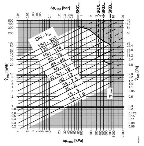
Δp<sub>max</sub> = Maximum permissible differential pressure across the valve (mixing: port A-AB, B-AB, diverting: port AB-A, AB-B), valid for the entire actuating range of the motorized valve
