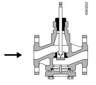
Depending on the nominal size, a guided perforated or slot plug is used that is directly connected to the valve stem.
