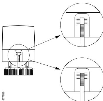
In this position, the actuator is de-energized: the actuator stem is retracted and the valve is closed.
