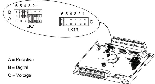
Refer to the controller's 'Controller Definition Drawing' in VisiSat for a picture of the required UI jumper settings for the controller. Factory default configuration is shown in the following table. If an input is not used, leave jumper in the default position.
