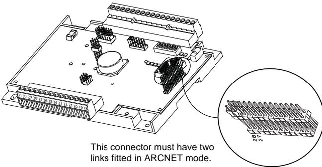
4. Connect the controller with other ARCNET devices in a device-to-device fashion. Do not use wiring trees or stubs.
