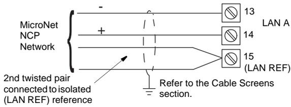
Ground the NCP wiring screen **at one end of the cable only**, e.g. at the earth terminal of an MN50-MI-NCP.
