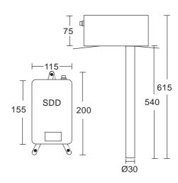
End resistor 2,2 KW (included in the control unit package)
