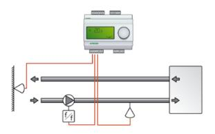
The output signal will increase when the pressure signal falls below the setpoint value.
