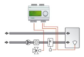
Humidification and dehumidification can be used simultaneously. A neutral zone can be set between humidification and dehumidification.
