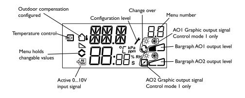
All the configuration menus lie in the 10-seconds level. This level is accessed from the Base Display by clicking and holding the encoder knob for 10 seconds.
