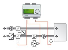
For control mode "Supply air temperature control" you need only one sensor, "Supply air sensor" on AI1
