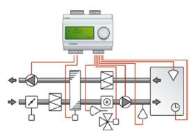
For control mode 3, "Cascade connected room / Exhaust air temperature control" you also need 2 sensors, "Supply air sensor" on AI1 and either "Room sensor" or "Exhaust sensor" on AI2.
