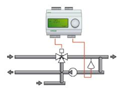
For this control mode you need a single sensor, "Supply water temperature" on All
