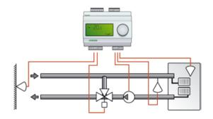
For this control mode you need two sensors, GT1 "Supply temperature" on AI1 and GT2 "Outdoor sensor" on AI2.
