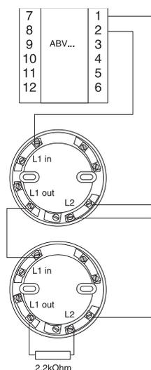
**N.B.** The end resistor must be connected to the last detector in the loop.
