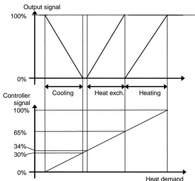
It is also possible to split one of the three analogue outputs into two equal parts to give a fourth output sequence for temperature control.
