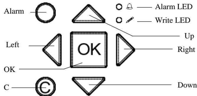
There are seven buttons: 4 arrow buttons which will be called UP, DOWN, RIGHT and LEFT. The menus in the Corrigo E are organized in a horizontal tree structure. The UP / DOWN-buttons are used to move between menus at the present menu level. The RIGHT / LEFT buttons are used to move between menu levels. When changing parameters the UP / DOWN buttons are used to increase / decrease the value of the parameter and the RIGHT / LEFT buttons to move between digits within the parameter.
