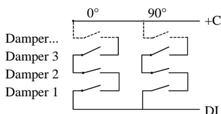
When the test cycle is initiated, the output *Fire dampers* will be activated and the dampers will begin to move. Within the set time (90 sec) the signal on the *input Fire damper end-switch monitoring* must change to indicate that the dampers have left their normal positions. If not an alarm will be triggered.
