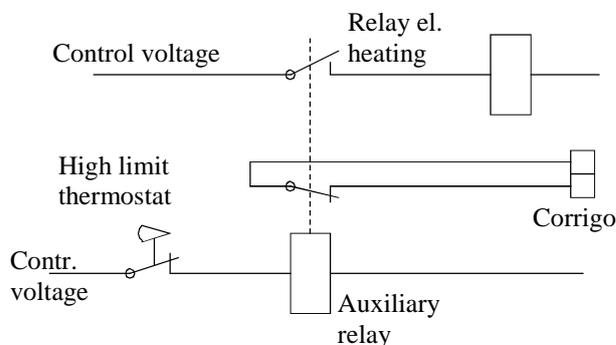
Wiring suggestion high temp limit when using electric heating. Contacts drawn inactivated.
