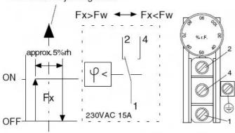
Fx air relative humidity (process value) Fw humidity adjusted at a set value
